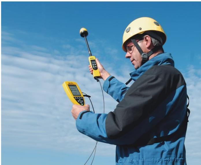
*Probe extension using an optical cable: The NBM-550 acts as controller and displays the results. The smaller NBM-520 acts as the optical probe interface. Both devices can also be used separately as measuring devices when fitted with probes.*
